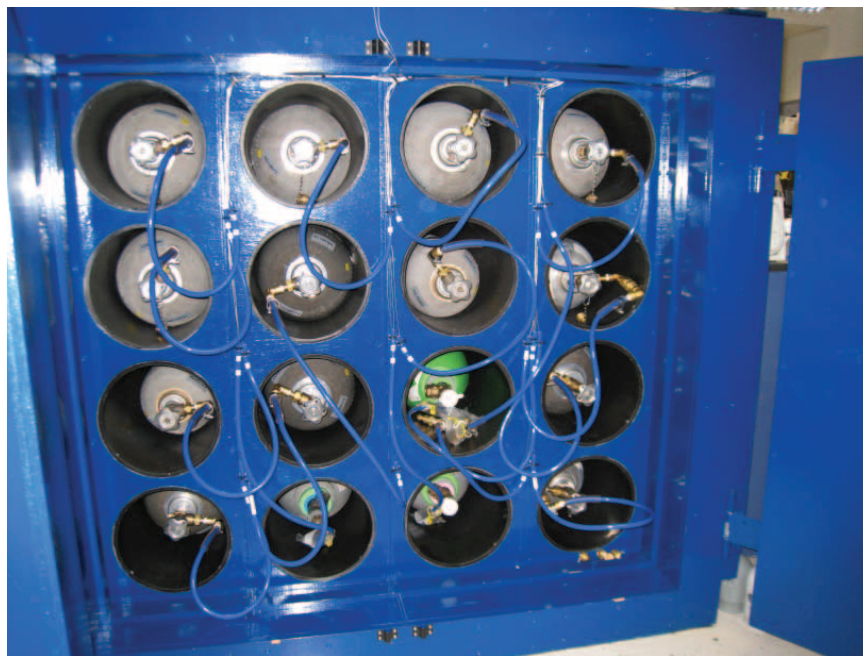
Fig. 8. Multiple array of precalibrated compressed air tanks for calibration of CO 2 intake. (© Marcos Lutyens. Photo © Francis Ware.)
